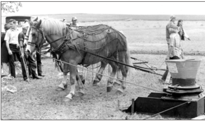
Bill Shold demonstrates a restored horse-powered sweep grinder once used by his grandfather.
