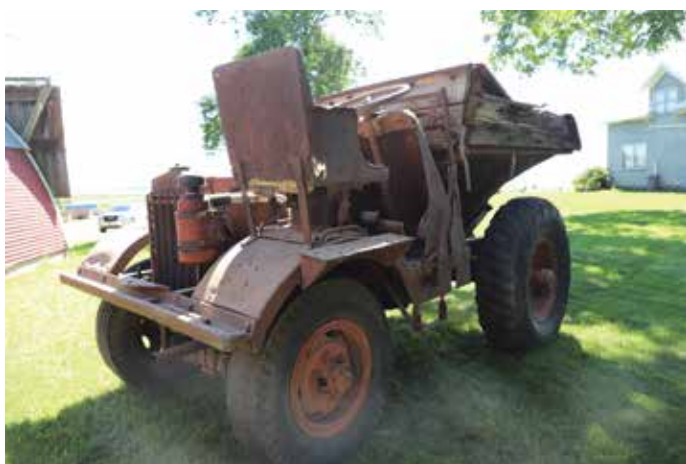
From 1934, a Koehring Wheel Dumptor model 70-5 with a Case L engine.
