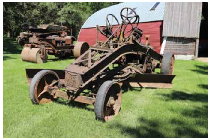
From the mid-1930s, a Wehr One Man Road Grader built on a Case model CI.
