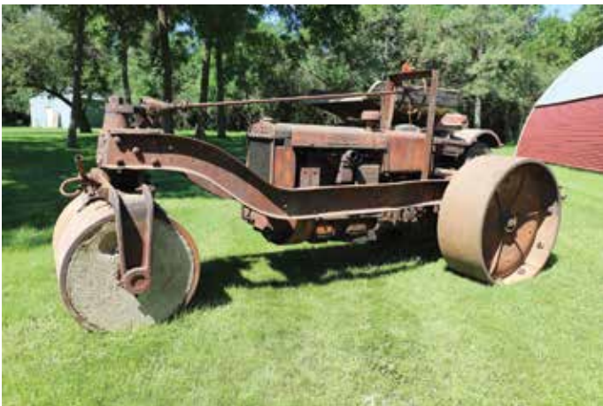
A 1932 Wehr road roller mounted on a Case model C tractor.
