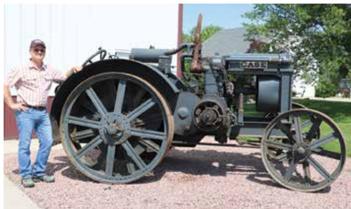
Steve Wacker is the proud owner of this Case crossmotor. The Case 25-45 weighs 10,065 pounds. It is 90 inches tall, 153 inches long and 82.5 inches wide.
