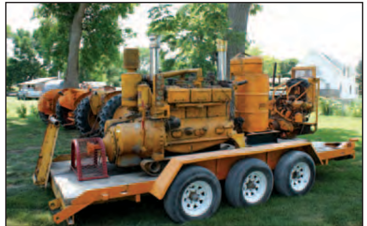
A Model 1210 that will come to the show. It has two 605 engines and was typically used for irrigation. Also on the trailer is a self-propelled V4 engine to use with the Uni-Harvester.
