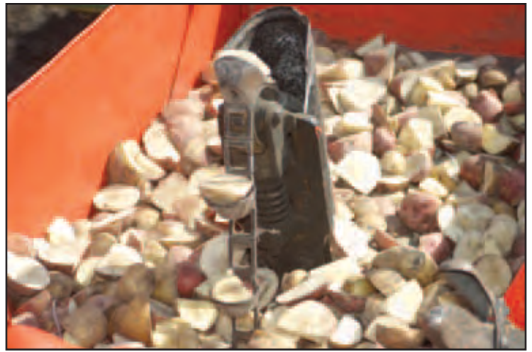
The cut seed potatoes fall into the small elevator cups which turns and plants one at the designated intervals.
