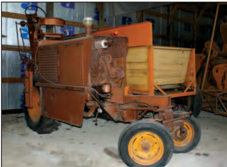
A Uni-Harvester from the 1950s. It could use the same engine for all applications. They system was later bought by New Idea.
