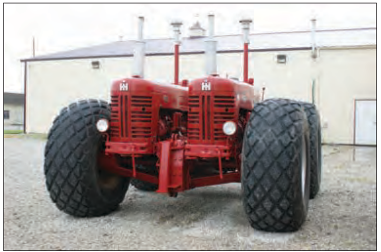
This one-of-a-kind tractor is now on display at Farmall Land. It is a twin drive 400 IHC Diesel. There was only one assembled and patented around the year 1956 by Garrett Mfg., in Enumclaw, Wash. It was a very large rubber-tired farm tractor at that time, weighing 15,380 pounds. The 400 IHC Diesel spent 30 years farming. It is on loan at Farmall Land for the rest of this year.
