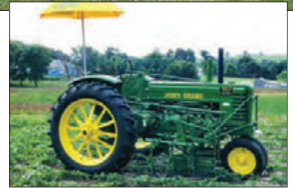
Russell's 1939 John Deere B with a 200 series cultivator featuring the Quick-tatch.
