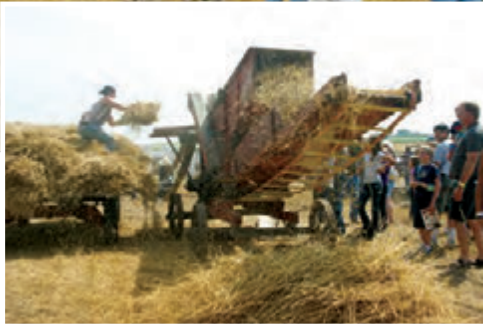
Horses power the hand-fed threshing machine.
