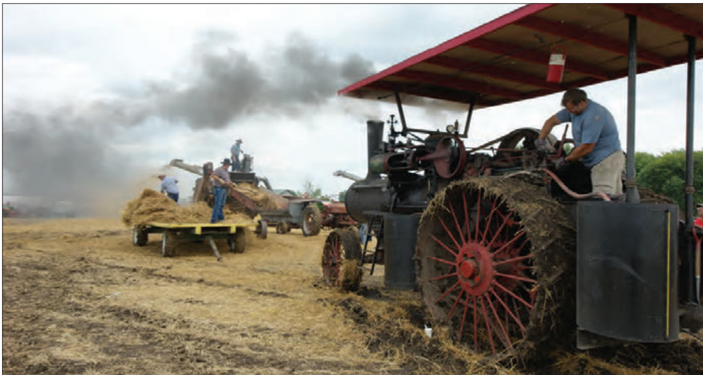
Threshing with steam power is always a popular attraction out in the field. Pictured is Bill Collins operating his 1918 Advance Rumely. The engine weighs 12-1/2 tons and has 60 horse-power on the belt and 20 horse-power on the draw bar. Each year the Threshermen plant about 22 acres of wheat at the show site. About one-third of the field is left standing for field activities while the remainder is harvested two weeks before the show and is then used for threshing demonstrations during the show.
