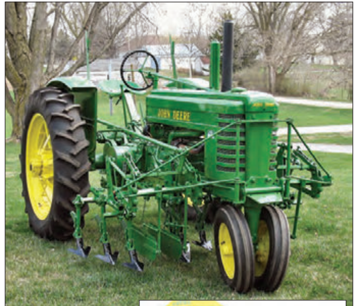
Russell's 1939 John Deere B with a 200 series cultivator featuring the Quick-tatch.
