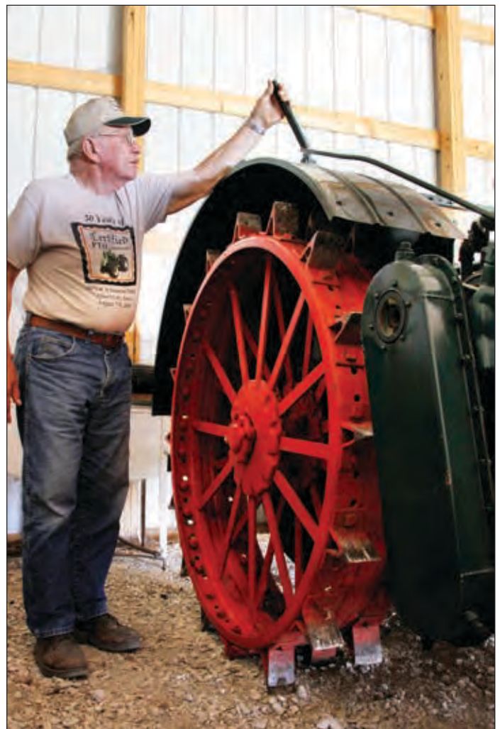
Lussman shows off the control lever for the "live power," a rare feature on this 1929 Hart-Parr 18-36.
