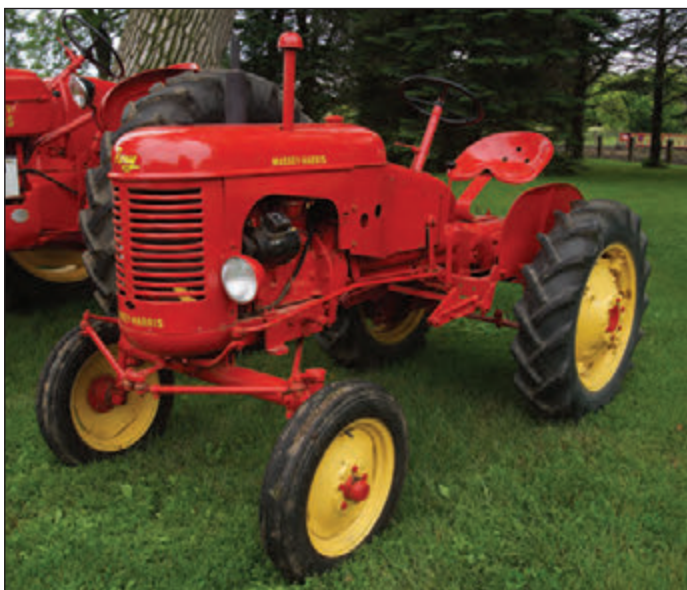
Paul bought this Massey Pony in Lansing. In 1947, Massey introduced the Model 11 Pony tractor that was rated at 10 HP on the drawbar. It was designed for small operations and truck farms, and was produced for 10 years.
