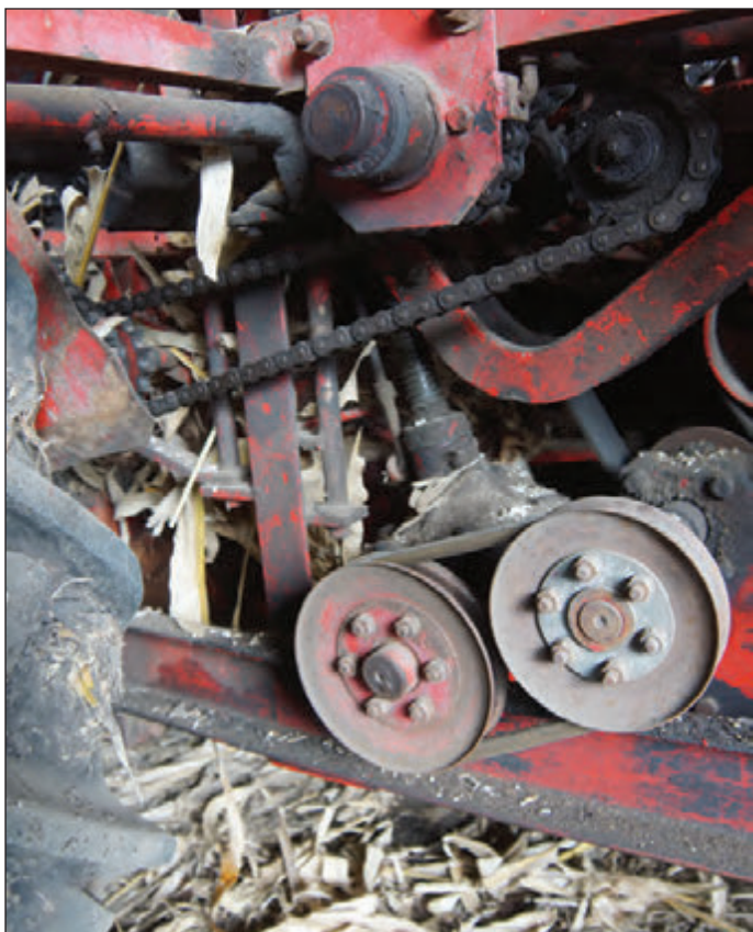
The Massey corn picker is driven with a series of chains and gears.
