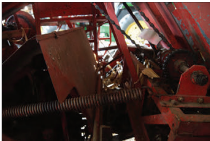
According to Brice, this model of corn picker was known for having a lot of fires as the husked corn travelled near to the engine.
