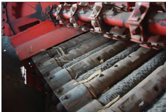
The 10-roll husking bed in the Massey corn picker.
