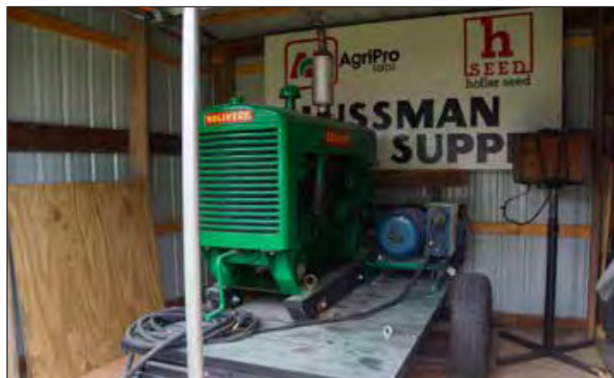
The Oliver 88 Power unit with a 225,000 watt generator.
