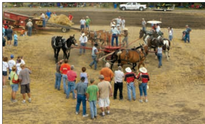
A demonstration of horse-powered sweep giving power to a hand-fed thresher at the show.
